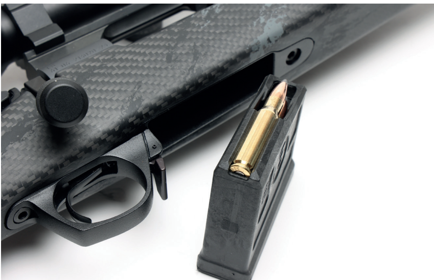
The five-shot, AICS-compatible, single-stack magazine in polymer works a treat
